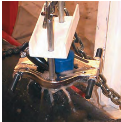
FIGURE 4 PULL-OUT TEST POLYETHYLENE PIPE
