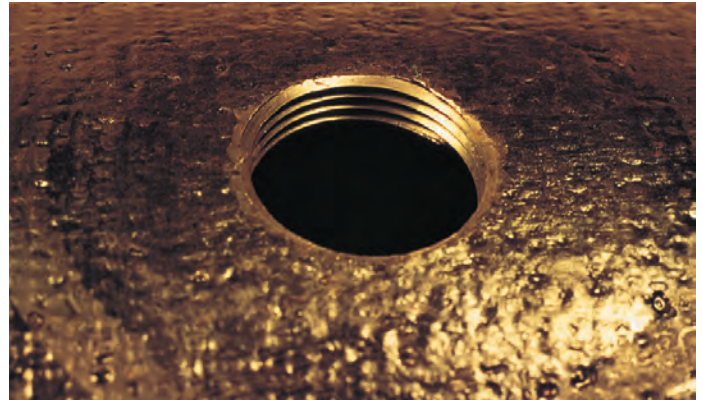
FIGURE 3 PULL-OUT TEST DUCTILE IRON PIPE
