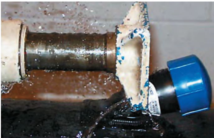
FIGURE 6 CANTILEVER LOAD TEST – POLYETHYLENE PIPE
