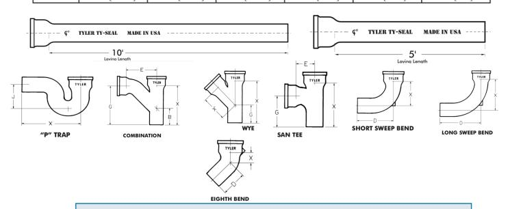
Extra Heavy Soil Pipe & Fittings are manufactured in accordance with ASTM A74.
