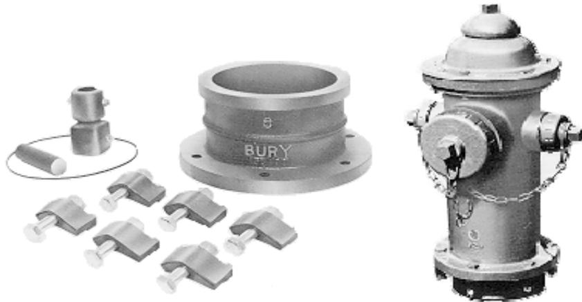
**Type:** Compression type, opening against line pressure. Main valve on Traffic Model will remain closed should hydrant be broken off by traffic accident.
