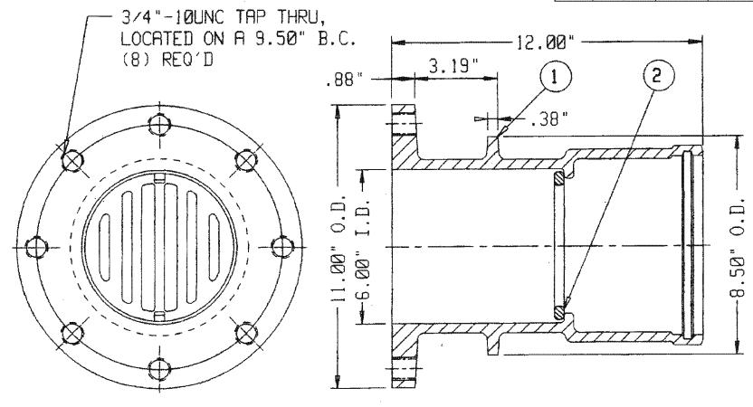
Can be extended to any length by using C900 P.V.C.
