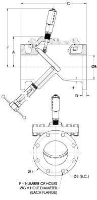
END FLANGES CONFORM TO ASME B16.1 CLASS 125
