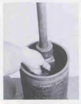
7 Remove hex nut (32) and bolt (31) from stem coupling (35). Lift off upper stem (36) and coupling.
