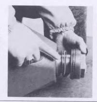
2 Remove thrust nut (4) by turning C.W. Remove operating nut (1) by turning C.C.W. on O.L. hydrants. C.W. on O.R. hydrants.
