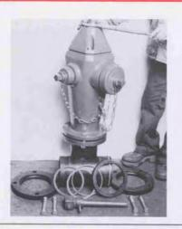
1 Remove thrust nut (4) by turning C.W.
