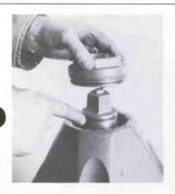
9 Lubricate and install o-ring (45) in groove in operating nut. Slide thrust nut (4) over operating nut and thread into cover.
