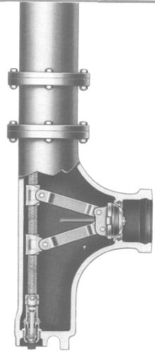
MAIN VALVE CLOSED Drain Valve Open
