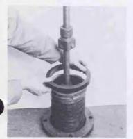
10 Place one lower flange (7) over standpipe, making sure that beveled portion is facing up. Replace retaining ring (26) in standpipe groove.
