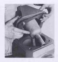
6 Thoroughly clean gasket surfaces on nozzle section (3) and cover (2). Lubricate and install orings (13) in grooves in cover. Slide upper stem sleeve (49) in cover. Place gasket (10) on top of nozzle section and carefully lower cover into place. Install cover bolts (9) and tighten securely.
