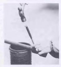
4 Drive out pin (34) and remove broken piece of coupling (35) from upper stem. Remove nut (32) and bolt (31). Pull broken coupling from lower stem.
