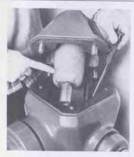
Check o-rings (13) and (43). Replace if worn or damaged. Install upper stem sleeve (49).
