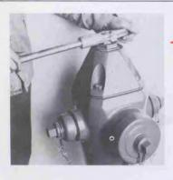
10 Open and close hydrant valve to make sure that it operates smoothly and easily. Turn on water in main and check hydrant valve for leakage by listening at open nozzle.
