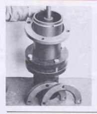
14 For one piece break flange: place break flange (50) with beveled portion up, over extension and place retaining ring (26) in upper groove of extension. For split break flange: install retaining ring (26) first. Break flange will be installed later.
