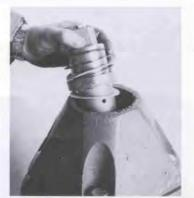
8 Screw operating nut (1) onto upper stem with Delrin bearing (42) in place. Install another Delrin bearing (42) between two races (5) on operating nut.
