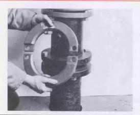
16 Set nozzle section in place on extension. Rotate break flange to line up holes and bolt in place. Torque bolts to 120 ft. lbs. keeping a uniform space between flanges. Note: For two piece break flange: Install break flange (beveled side up) at this time—tighten bolts at overlap of ring first.
