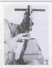
19 Install hex stop nut (12) and tighten securely with combination tool.
