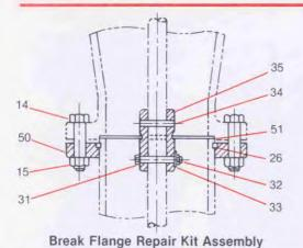
Break Flange Repair Kit Parts List
