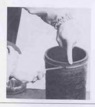
1 Remove retaining ring (26) from groove in standpipe. Place new retaining ring (26) in standpipe groove.
