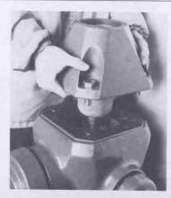
9 Place gasket (10) on top of nozzle section. Slide cover (2) over stem and bolt in place.
