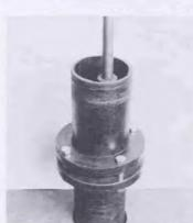
12 Place retaining ring (26) in lower groove of stand-pipe extension (53) (lower groove 1¼ " from end of extension), and place extension on standpipe. (Make sure gasket remains in place).
