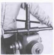
7 Unscrew seat ring by turning counterclockwise approximately six full turns.
