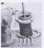
6 Remove retaining ring (26) and break flange (50).
