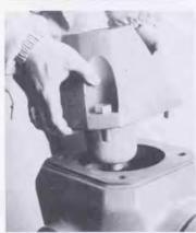
6 Remove cover bolts (9) and remove cover (2) from nozzle section (3).
