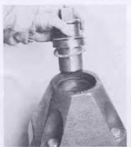
11 Screw operating nut (1) onto upper stem with lower Delrin bearing (42) in place. Install remaining Delrin bearing (42) between two races (5) on operating nut.
