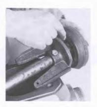
2 Install seat rubber (24) in place and screw lower valve plate (25) onto lower stem (37). Tighten with approximately 50 ft-lbs torque.
