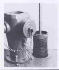
5 Remove four hex nuts (15) and (14). Lift nozzle section over stem and lay aside.
