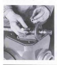
All gaskets and o-rings should be replaced when reassembling hydrant. Any other damaged or worn parts should be replaced as required.
