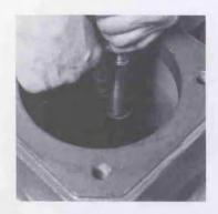
5 Lubricate and install o-ring (43) in groove in upper stem (36)
