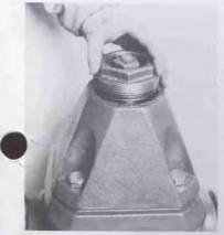
12 Slide thrust nut (4) over operating nut and tighten with 150 ft. lbs. torque.
