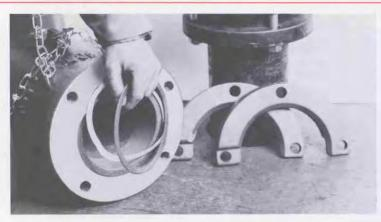
15 Thoroughly clean machined recess in bottom of nozzle section. Remove adhesive backing on new gasket (51) and insert into recess in bottom of nozzle section. Lubricate gasket which will allow nozzle section to be rotated to desired position before flange bolts are tightened.
