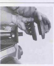
10 Unscrew lower valve plate (25) by turning counterclockwise and remove seat rubber (24).
