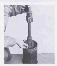
8Assemble new round barrel stem coupling (35) to the lower stem (37).
