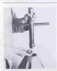
10 Thread hex stop nut (12) onto upper stem and tighten securely with combination tool.
