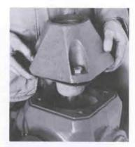
5 Remove cover bolts (9) and lift off cover (2).
