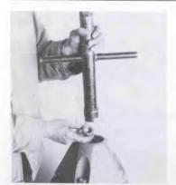
7 Install hex stop nut (12) and tighten with combination tool.
